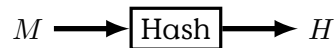
Figure 4.19: Hash function with input message M and output hash value H . (See [Aumasson18seriouscrypto])
